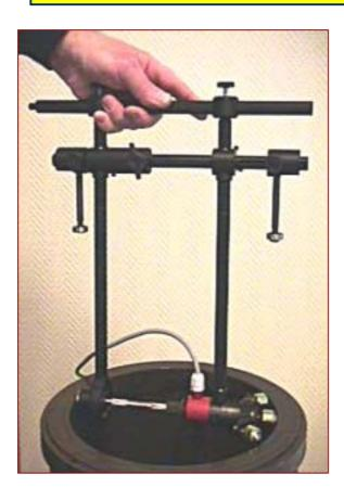
The Ovality Kit is an <u>accessory</u> to the DI-4C/CR Deflection Indicators, primarily designed to measure cylinder liner ovality and for wear comparison at bore diameters 180 – 600 mm and stroke up to 870 mm. This aluminium jig may be modified to take measurements in other applications as well.
